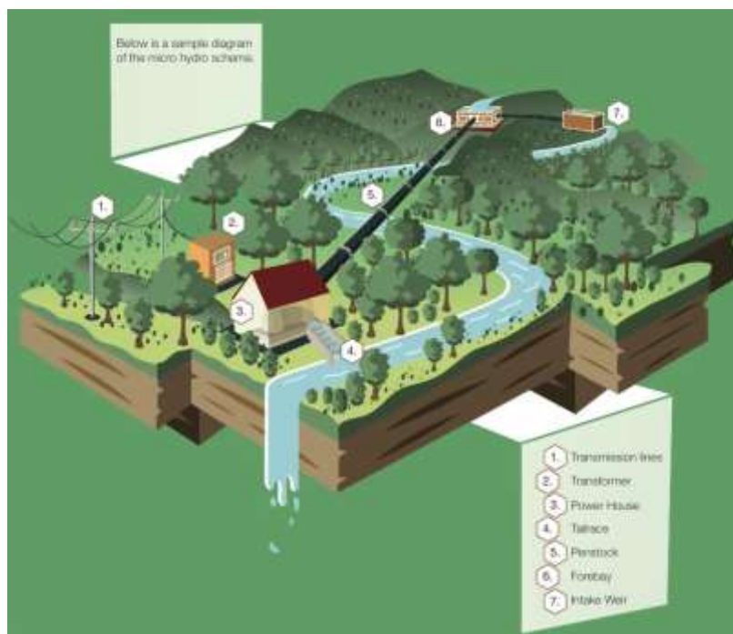
Figure 1. Microhydro Power Plant Scheme
